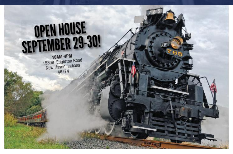
She weighs 404-tons, stands 16 feet tall, and can go 80 miles an hour. Steam locomotive no. 765 has been rocketing through the Midwest as a one-of-a-kind time machine and ambassador for Fort Wayne since being restored in 1979.
