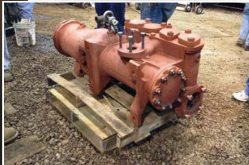
Looking not unlike an organ transplant, the water pump after returning from Chattanooga, Tennessee after being re-machined prior to the start of the season.
